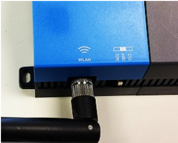
Figure 1 Antenna and switch location on enclosure
